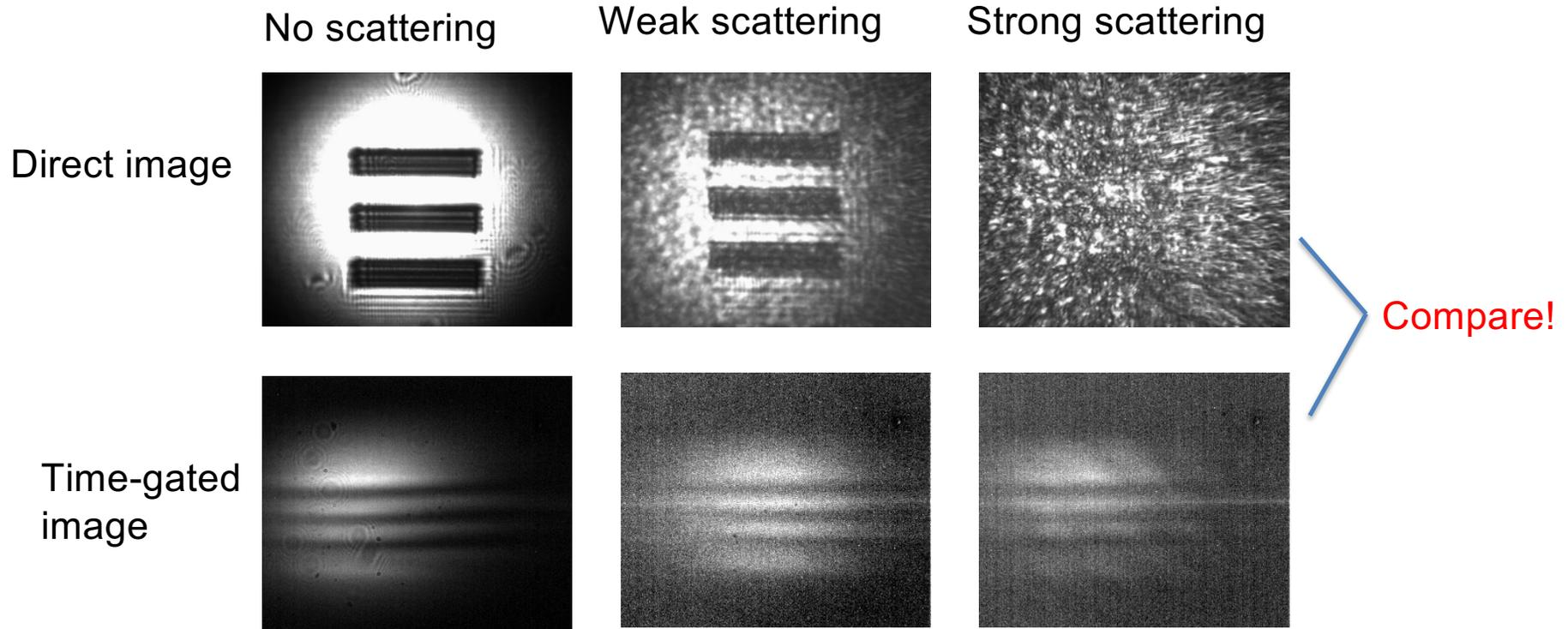
Need material with a strong, fast nonlinear optical response to construct gate. Use ITO.
