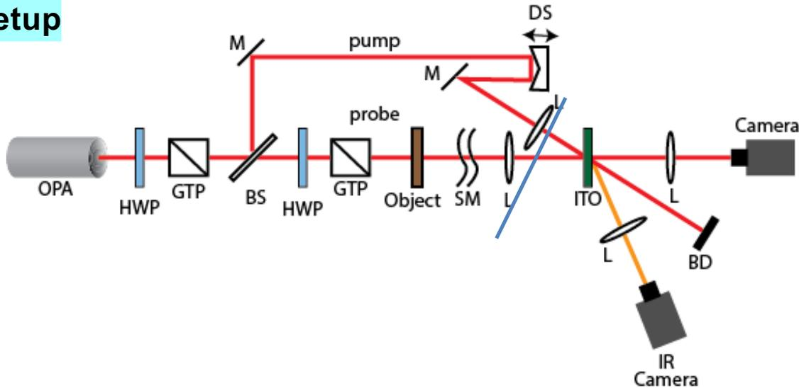
Probe transmission shuttered by pump pulse in a “Kerr gate.”
