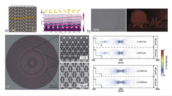
**FIG. 1.** Metasurfaces for wavefront control. (a) Generalized laws of refraction for beam steering through phase gradients (reproduced with permission from Yu *et al.*, Science **334**, 333 (2011). Copyright 2011 AAAS,<sup>5</sup> (b) metasurface holograms with high efficiency (from Ref. 20); (c) multi-wavelength, polarization-insensitive metalenses (from Ref. 21). All images are reprinted (adapted) with permission from the respective Journal and copyright remains with the original publisher.
