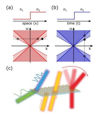
**FIG. 28.** Scattering of light traveling in the x direction at a (a) spatial and (b) temporal interface can be illustrated with dispersion diagrams, where the full and dashed lines denote the dispersion cones for the two media. (c) An illustration of a device that combines advanced structuring of both spatial and temporal inhomogeneities to provide dynamic control over the momentum and frequency of scattered light, adapted from Ref. 48. Copyright remains with the original publisher.
