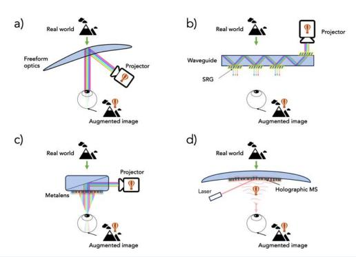
FIG. 16. Four AR architectures: (a) freefrom optical combiners; (b) waveguide combiners with metagratings; (c) prism combiners with a metalens; (d) holographic metasurface combiners. (a)–(c) use full-color projectors to generate virtual image; and (d) uses plain laser beams and the virtual image is encoded in the metasurface.
