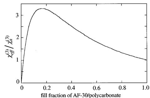
FIG. 1. Predicted enhancement of the electro-optic response plotted as a function of the fill fraction of the doped-polycarbonate constituent of the layered composite material.
