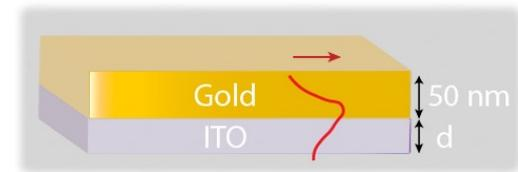
Fig. 1: Diagram of the bi-film.
