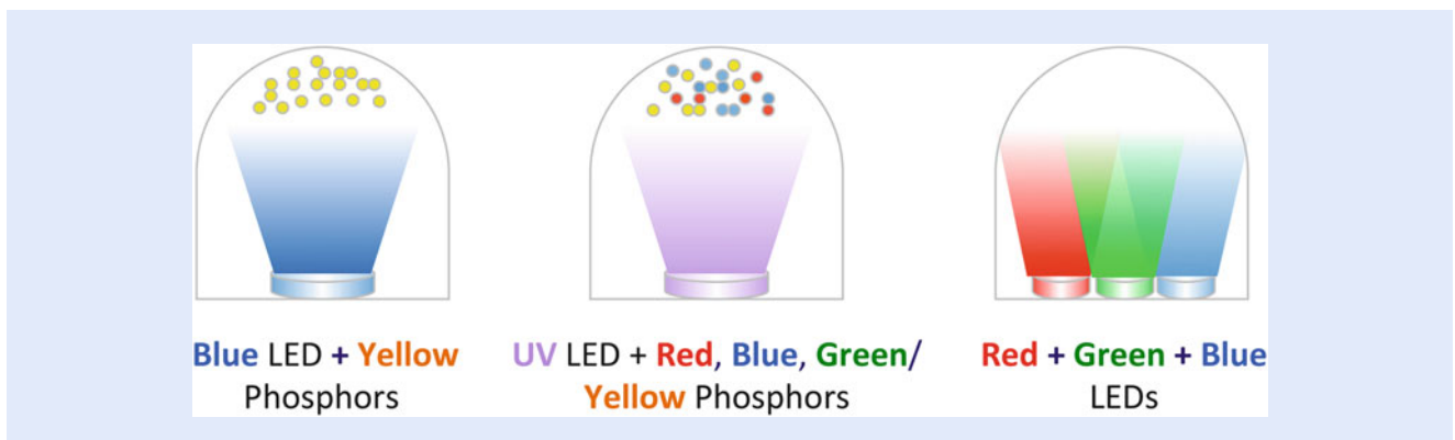
Fig. 5.16 Illustration of white light generation using phosphor method (blue/UV LEDs + phosphors) and using RGB method (Red + Green + Blue LEDs)
