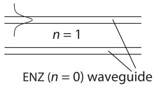
Mode of upper waveguide beams into the lower waveguide even for large separation
