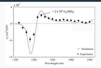
The material exhibits extremely large n2 over a broad spectralrange. The magnitude of the on-resonance value is 7 orders of magnitudelarger than that of SiO2.Alam, Schulz, Upham, De Leon and Boyd,
