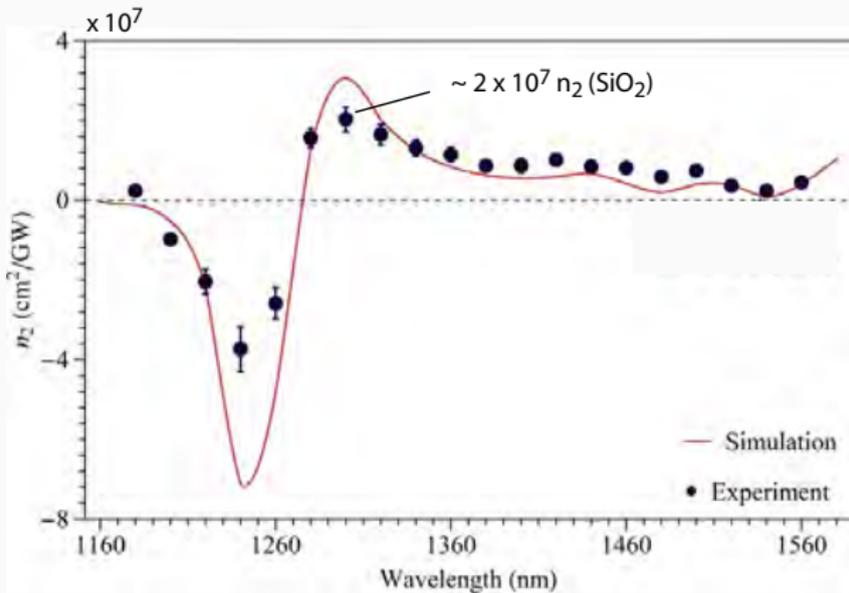
The material exhibits extremely large  $n_2$  over a broad spectral range. The magnitude of the on-resonance value is **7 orders of magnitude larger than that of  $\text{SiO}_2$** .
