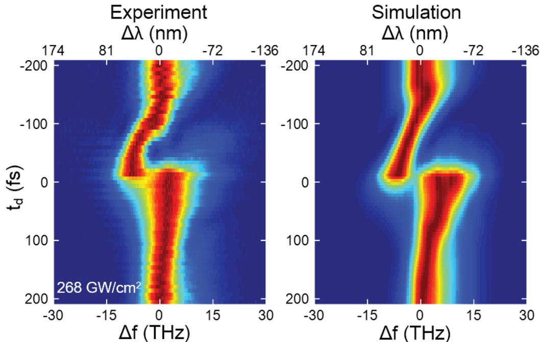
Probe phase and amplitude are measured by frequency-resolved optical gating (FROG)
