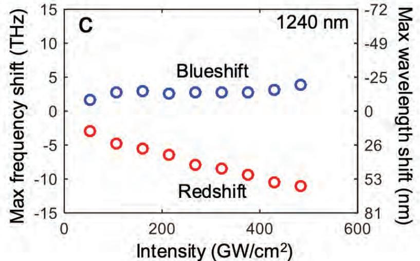
The wavelength shift can be controlled by the pump intensity and the sign of the time delay.
