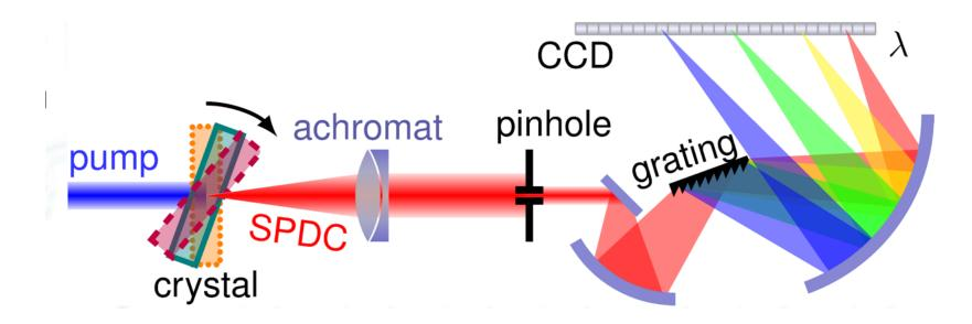
We rotate the crystal to vary the phase matched wavelength. We end up with data that looks like this.
