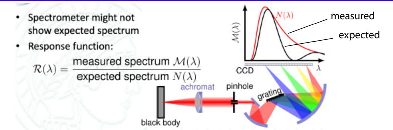
Laboratory measurements of the response function
