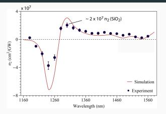
The material exhibits extremely large  $n_2$  over a broad spectral range. The magnitude of the on-resonance value is 7 orders of magnitude larger than that of  $SiO_2$ .
