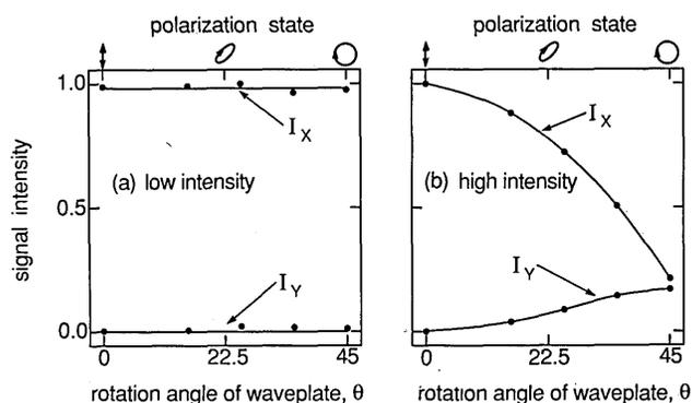
Fig. 3. Intensity of each polarization component plotted as a function of the degree of polarization distortion introduced into the probe wave. (a) For low pump intensities ( $0.16I_{\text{sat}}$ ), the effects of the polarization distortion are removed essentially completely ( $I_x$  is independent of  $\theta$  and  $I_y \ll I_x$ ). (b) For high pump intensities ( $1.7I_{\text{sat}}$ ), severe degradation of the VPC is observed ( $I_x$  and  $I_y$  are comparable and depend on  $\theta$ ).
