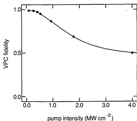
Fig. 4. Fidelity of the VPC process, quantified by the ratio  $I_x/(I_x + I_y)$  (i.e., the ratio of the intensity of the proper polarization component to the total output intensity), plotted as a function of the intensity of one of the pump waves. The waveplate in Fig. 1(b) has been oriented to produce circular polarization.
