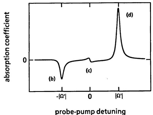
Fig. 2. The probe absorption spectrum as modified by the intense pump-laser field for  $T_2/T_1 = 2$ ,  $\Omega T_2 = 20$ , and  $\Delta T_2 = -5$ . (b)–(d) Correspondence between the three spectral features and the transitions illustrated in Fig. 1.
