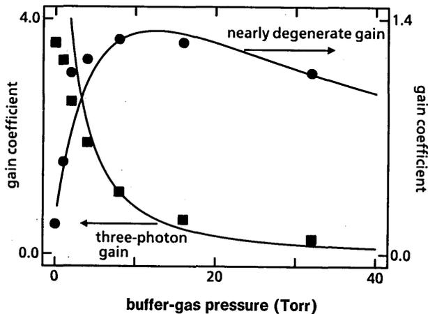
Fig. 5. Measured peak gain coefficient for the three-photon feature (squares) and the nearly degenerate feature (circles) versus helium buffer-gas pressure. The solid curves are fits of Eqs. (11) and (4)–(9), respectively, to the data, with Eq. (15) relating the buffer-gas pressure to the dipole-dephasing time  $T_2$ .
