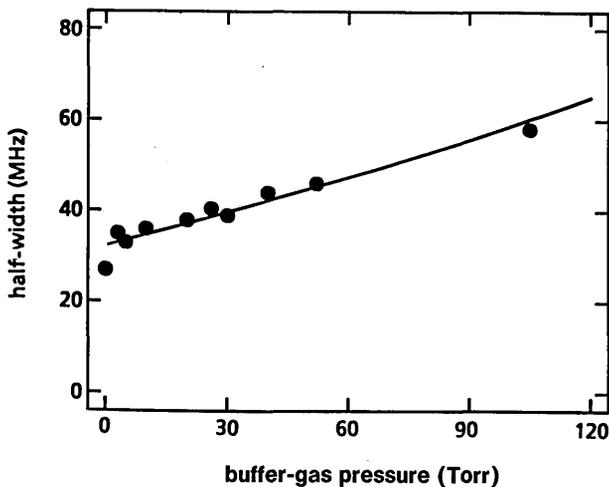
Fig. 6. Half-width of the nearly degenerate feature versus helium buffer-gas pressure. The experimental pump detuning from resonance for the zero-velocity group of atoms is approximately  $-6.5$  GHz. The solid line is a theoretical fit to the data taking  $\Delta_0/\Omega = -5$  and a beam-crossing angle of  $1.6^\circ$ .
