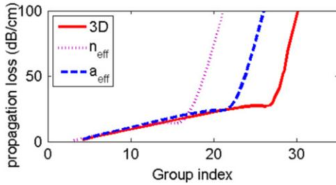
**Figure 3.** Plot of propagation loss against group index. The true behaviour, 3D simulations, is better approximated by the effective period method ( $a_{\text{eff}}$ ) rather than the EIM ( $n_{\text{eff}}$ ). However both 2D simulation methods underestimate the threshold for the rapid increase of propagation loss.
