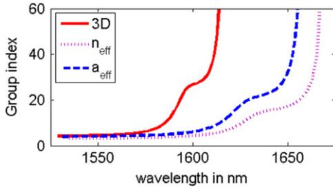
**Figure 2.** Group index for a dispersion engineered waveguide, as calculated by the different simulation methods. The true 3D simulations, the EIM ( $n_{\text{eff}}$ ) and the effective period method ( $a_{\text{eff}}$ ).
