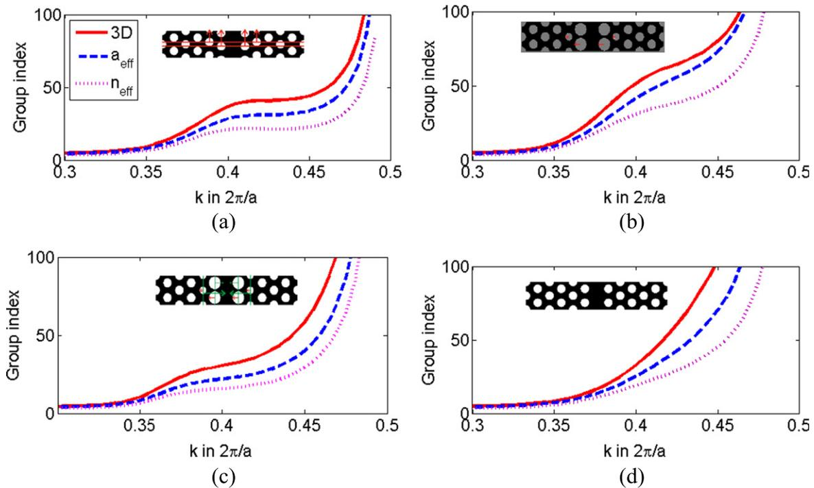
**Figure 5.** Plots of group index against the wave-vector for other waveguide designs and sketch showing the engineering method: (a) holes shifted parallel to the waveguide [28] (b) silica-clad waveguide with radius variation [13] (c) combination of hole shift and radius reduction [29] and (d) a W1 waveguide [30]. In all cases the 3D results are better approximated by the effective period method ( $a_{\text{eff}}$ ) rather than the EIM ( $n_{\text{eff}}$ ).
