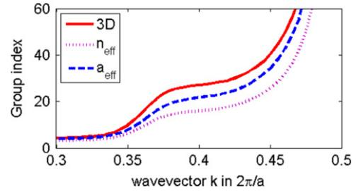
**Figure 4.** Plot of the group index against the wave-vector. The true 3D value is better approximated by the bulk index 2D calculation ( $a_{\text{eff}}$ ) than by the EIM ( $n_{\text{eff}}$ ).
