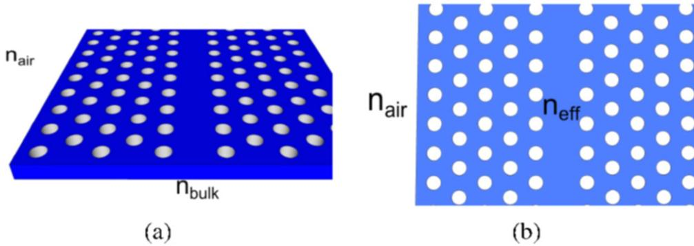
**Figure 1.** (a) 3D sketch of a photonic crystal waveguide. (b) 2D adaptation of this waveguide as it would be treated with the effective index method (EIM), the bulk slab material index ( $n_{\text{bulk}}$ ) has been replaced with the slab mode effective index ( $n_{\text{eff}}$ ).
