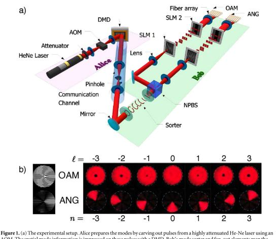
AOM. The spatial mode information is impressed on these pulses with a DMD. Bob's mode sorter and fan-out elements map the OAM modes and the ANG modes into separated spots that are collected by an array of fibers. (b) The alphabet. CCD images of produced light field profiles in two complementary spatial bases of OAM and ANG (d=7). The intensity profile of the modes are shown on the right. An example of binary holograms used for the generation of modes in each basis is shown on the left.
