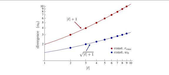
**Figure 2.** The divergence of an OAM beam obtained by keeping the  $r_{\rm rms}$  radius in the launch plane constant is larger than for an OAM beam obtained by keeping the Gaussian waist  $w_0$  constant. Moreover, the first scales as  $|\ell| + 1$  whereas the second scales as  $\sqrt{|\ell| + 1}$ . This log–log plot is given in units of the divergence angle  $\alpha_0 = w_0/\sqrt{2} z_R$  of a fundamental Gaussian beam. The lines serve purely as a guide to the eye.
