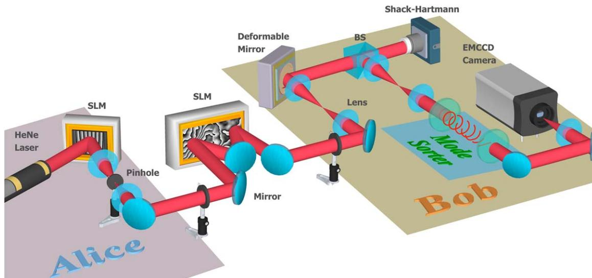
**Figure 4.** Alice sends a beam prepared in a specific orbital angular momentum state,  $\ell$ , to Bob. Bob receives the beam after propagation through a channel representing a 1 km turbulent path. The beam is (optionally) corrected using a deformable mirror and sent to a sorter to make a measurement of the of the orbital angular momentum spectrum of the beam.
