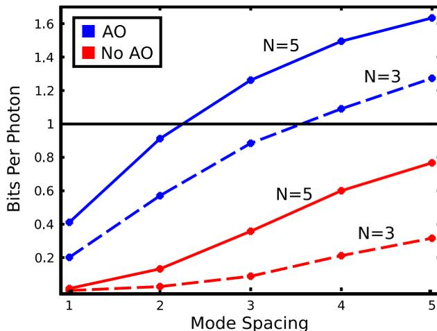
**Figure 7.** Measured channel capacity as a function of the spacing between OAM modes used for communication.
