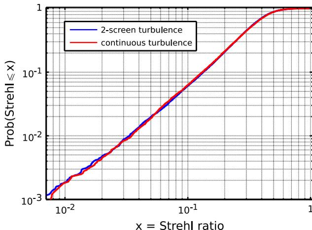
**Figure 2.** Cumulative distribution function (CDF) of the Strehl ratio for a thick turbulent path represented by ten Kolmogorov phase screens (red line) and its equivalent two-phase screen solution (blue line).
