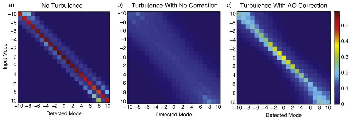
**Figure 5.** Measurement of the crosstalk in the channel represented by the conditional probability matrix,  $P(d|s)$  for three cases: (a) no turbulence, (b) with turbulence, and (c) with turbulence and adaptive correction.
