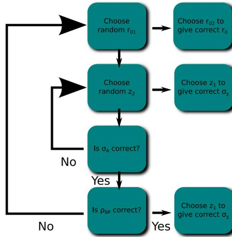
**Figure 1.** Procedure used to compute Fried's parameters and positions of the two thin phase screens needed to reproduce  $r_0$ ,  $\sigma_\chi$ ,  $\sigma_p$ , and  $\rho_{bp}$  of the equivalent thick channel.
