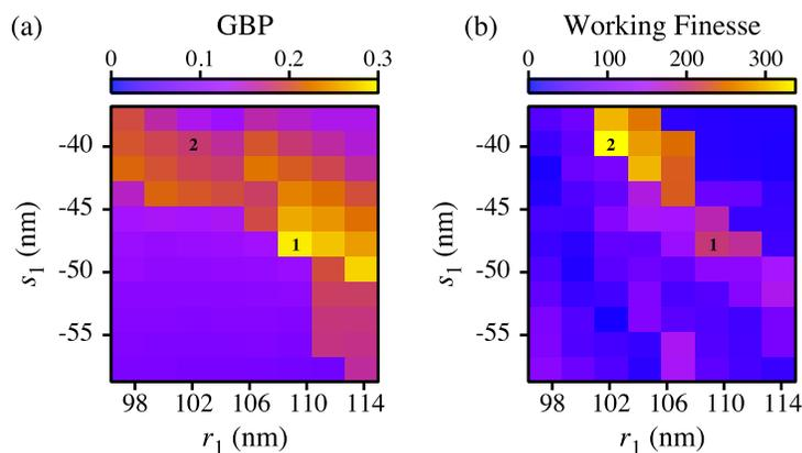
Fig. 2. Group index bandwidth product (a), and working finesse (b) of PhCWs for different values of the radius  $r_1$ , and lateral shift  $s_1$ , of the holes adjacent to the line defect. The designs corresponding to the maximum GBP and maximum  $\mathcal{F}_W$  are labeled ‘1’ and ‘2’, respectively.
