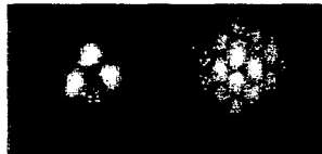
Fig. 1. Example of pattern formation as observed in the near (left) and far (right) fields of the sodium vapor cell.
