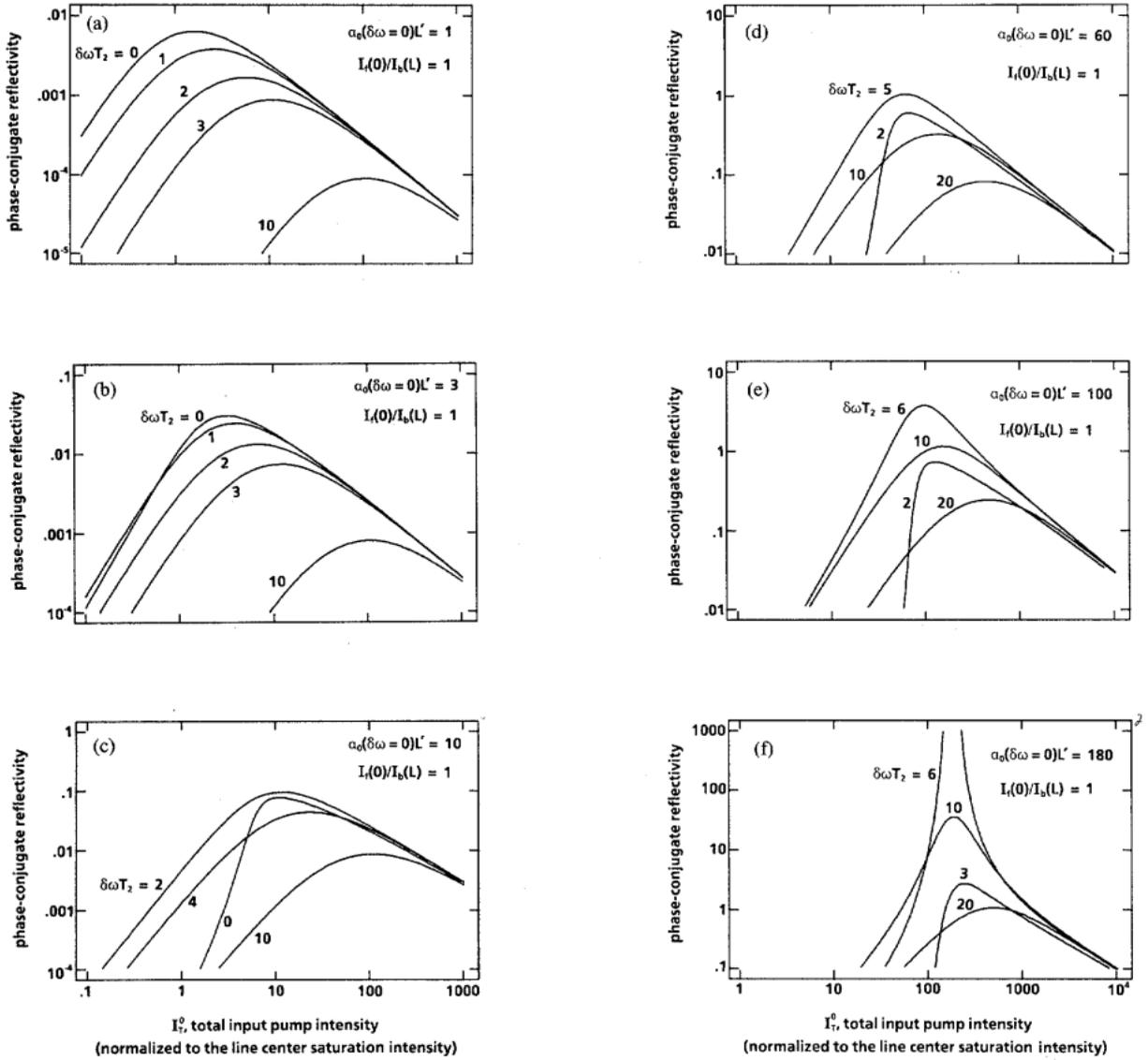
Fig. 2. Phase-conjugate reflectivity plotted as a function of the total input pump intensity normalized by the line-center saturation intensity. Equal input pump intensities are assumed. Each plot pertains to a different value of the unsaturated, line-center pump attenuation  $\alpha_0(\delta\omega = 0)L'$ , in the range 1.0 to 180, and in each plot several different values of the normalized laser detuning from line center,  $\delta\omega T_2$ , are shown.
