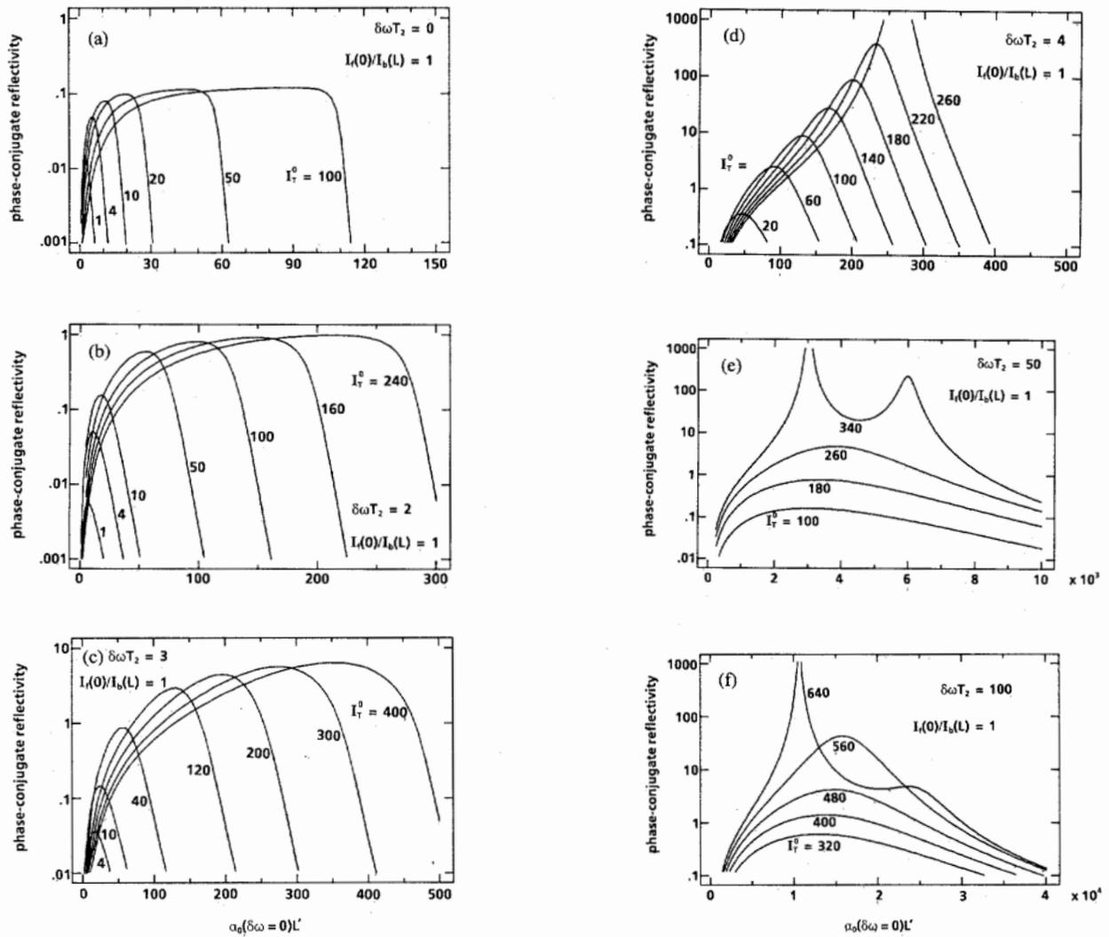
Fig. 4. Similar to Fig. 3, except that each plot pertains to a different value of the laser detuning from line-center,  $\delta\omega T_2$ , and in each plot several different values of the total input pump intensity normalized to the line-center saturation intensity are shown.
