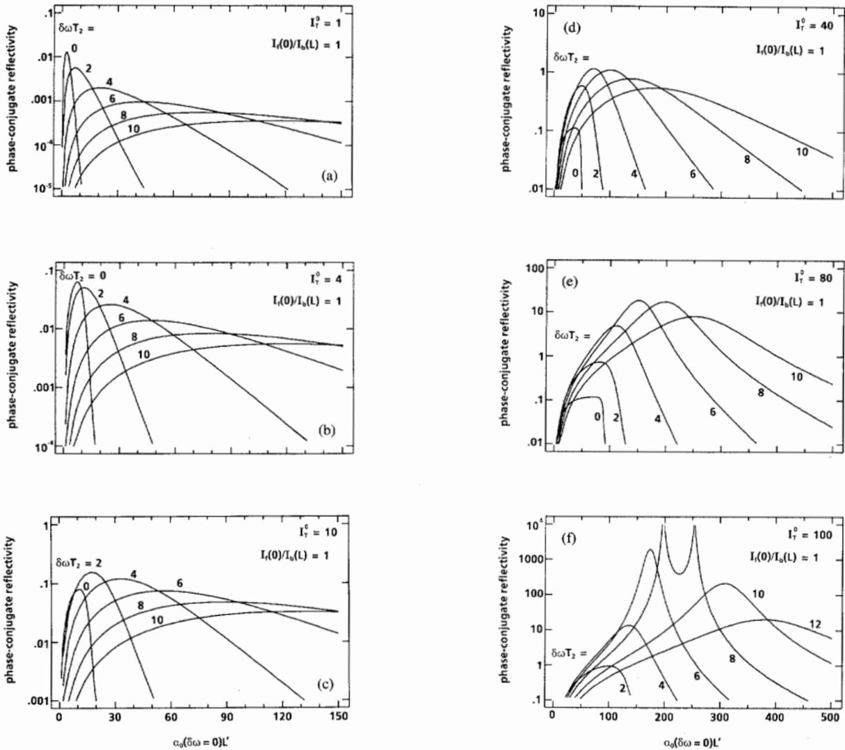
Fig. 3. Phase-conjugate reflectivity plotted as a function of the unsaturated, line-center, pump attenuation,  $\alpha_0(\delta\omega = 0)L'$ . Equal pump intensities are assumed. Each plot pertains to a different value of the total input pump intensity normalized by the line-center saturation intensity,  $I_T^0$ , in the range 1.0 to 100, and in each graph several different values of the normalized laser detuning from line-center,  $\delta\omega T_2$ , are shown.
