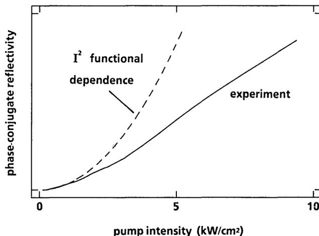
Fig. 3. Phase-conjugate reflectivity in arbitrary units versus pump intensity in each beam at a laser wavelength of 576 nm.
