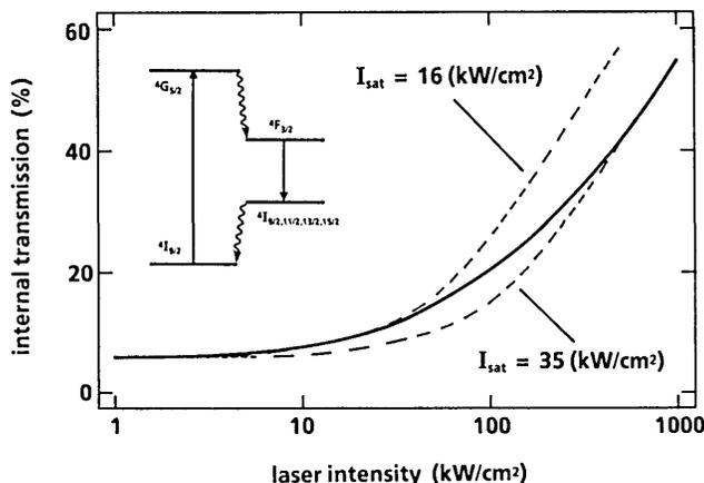
Fig. 1. Internal transmission of Nd<sup>3+</sup> beta" alumina versus laser intensity measured at a wavelength of 577 nm (solid curve). The dashed curves are theoretical predictions for an inhomogeneously broadened saturable absorber. The inset shows the relevant energy levels of Nd<sup>3+</sup>.
