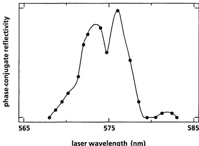
Fig. 2. Phase-conjugate reflectivity in arbitrary units versus laser wavelength at a pump intensity of  $10 \text{ kW cm}^{-2}$  in each beam.
