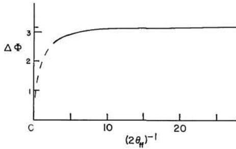
FIG. 4. The phase anomaly  $\Delta\Phi$  predicted by the heuristic argument described here is shown as a function of  $(2\theta_{ff})^{-1} \equiv f^\#$ . For large values of  $f^\#$ , the predicted phase anomaly agrees with the actual value of  $\pi$  radians. The broken portion of the curve corresponds to  $f^\# \lesssim 1$ , where the approximations used in the derivation are invalid.
