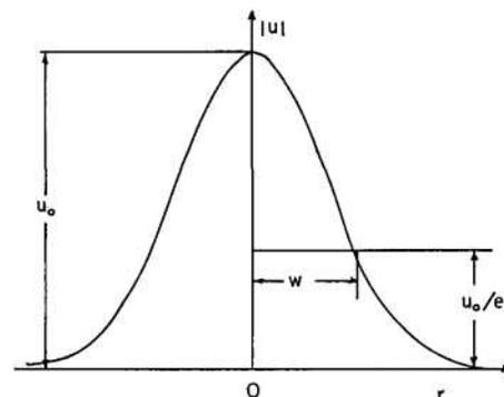
FIG. 1. Amplitude distribution of a Gaussian beam.
