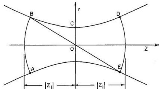
FIG. 3. The wave fronts  $AB$  and  $DE$  of a Gaussian beam are separated by the optical path length  $BCD$ . The difference between the path length  $BCD$  and the geometrical separation  $BE$  gives rise to the phase anomaly.
