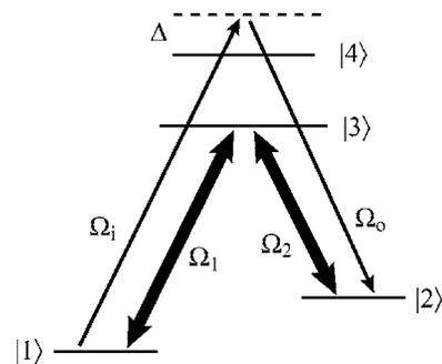
FIG. 1. The scheme for transfer of information from one frequency to another via coherent Raman scattering. The control fields  $\Omega_1, \Omega_2$  create quantum coherence between the ground states  $|1\rangle, |2\rangle$ . A weak input field  $\Omega_i$  scatters off this coherence, generating a new field  $\Omega_o$ . Any information imprinted on the input field is transferred to the scattered, output field.
