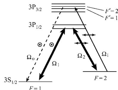
FIG. 3. The scheme for modulation transfer by coherent Raman scattering in sodium. A modulated input field  $\Omega_i$  scatters off the ground hyperfine coherence created by the control fields, creating a modulated field  $\Omega_o$ .
