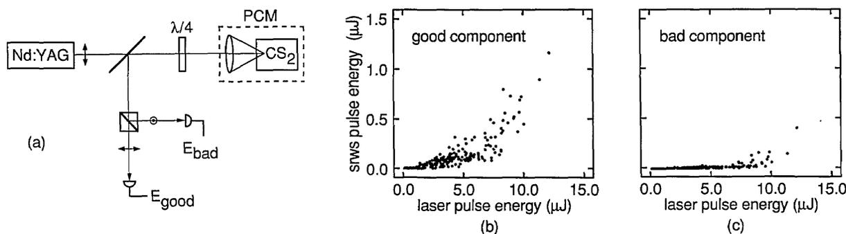
Fig. 3. Fidelity of polarization correction by SRWS. (a) Experimental setup. (b), (c) Energy in the good (b) and bad (c) components of the signal returned by SRWS plotted as functions of the laser pulse energy. For laser pulse energies less than 7  $\mu\text{J}$ , the polarization correction is essentially perfect.
