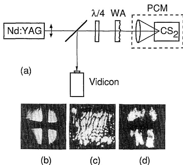
Fig. 1. Wave-front correction by SRWS. (a) Experimental setup. (b) Incident laser beam. (c) Laser beam after a double pass through the wave-front aberrator (WA) on reflection by a normal mirror. (d) The corrected beam after a double pass through the phase aberrator on reflection by SRWS.
