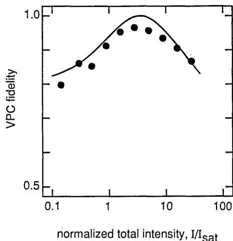
Fig. 4. Fidelity of the VPC process versus the normalized pump intensity. VPC fidelity is defined as the ratio  $I_g/(I_g + I_b)$ , that is, as the ratio of the intensity of the proper polarization component to the total output intensity. The circles represent experimental data plotted using  $I_{\text{sat}} = 100 \text{ mW/cm}^2$ , and the solid curve is calculated using the theory described in the text.
