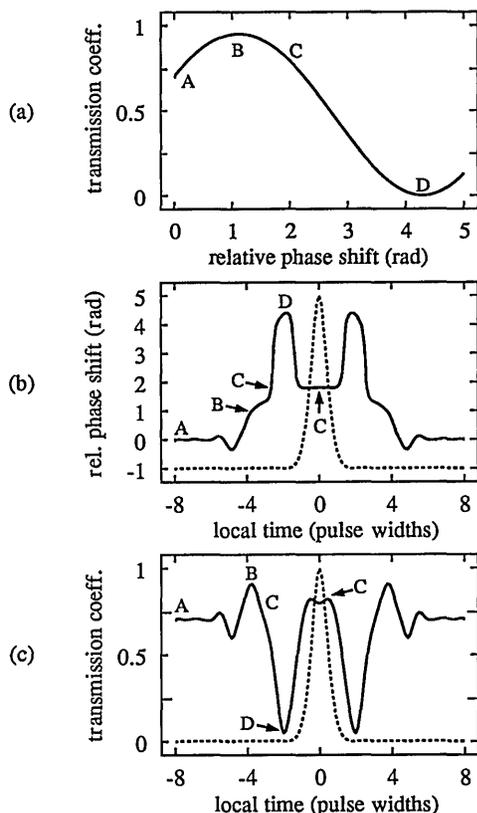
Fig. 3. Transmission coefficient of the nonlinear loop mirror as a function of the relative phase shift, as calculated from a scalar continuous-wave theory. (b) The relative phase shift and (c) the transmission coefficient of the nonlinear loop mirror as a functions of local time, as calculated numerically by use of a full tensor analysis. The pulse shape is shown by a dashed curve.
