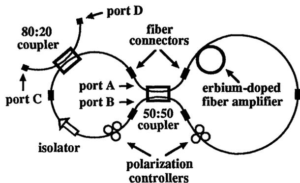
Fig. 1. Schematic of the fiber figure-eight laser.
