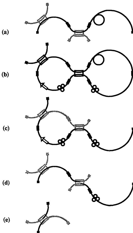
Fig. 2. Schematic of the experimental procedure for characterizing a figure-eight laser. (a) The birefringence in the bold section of the fiber is probed, (b) the laser is assembled and the average output powers and eigenpolarizations are measured for the characteristic modes of operation. (c)–(e) The birefringence in the bold sections of the fiber is measured as the laser is disassembled.
