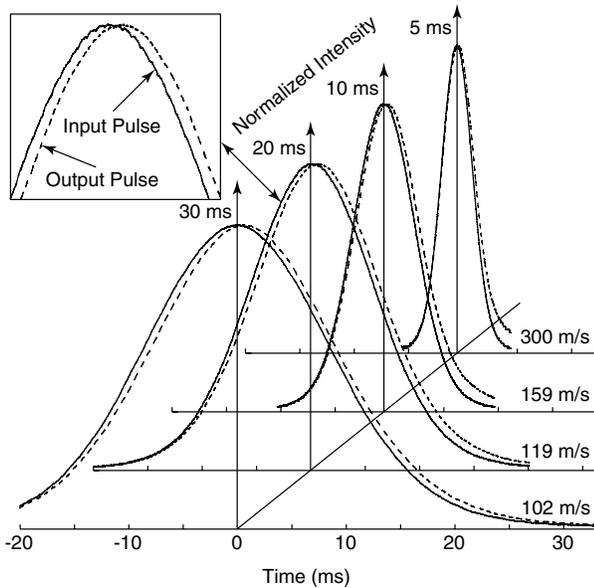
FIG. 4. The normalized input and output intensities of a 5, 10, 20, and 30 ms pulse. The corresponding average group velocities of the pulses are 300, 159, 119, and 102 m/s. The inset shows a close-up of the 20 ms pulse.
