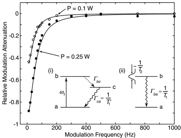
FIG. 2. The relative modulation attenuation  $A(\delta)$  with respect to the pump as a function of modulation frequency for input pump powers of 0.1 and 0.25 W. The solid lines represent the theoretical model of Eq. (10). The insets show the two coupling schemes discussed in the text.
