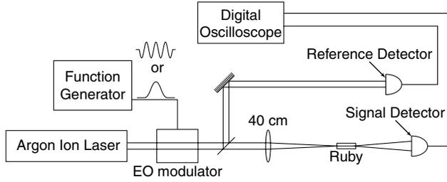
FIG. 1. The experimental setup used to observe slow light in ruby.
