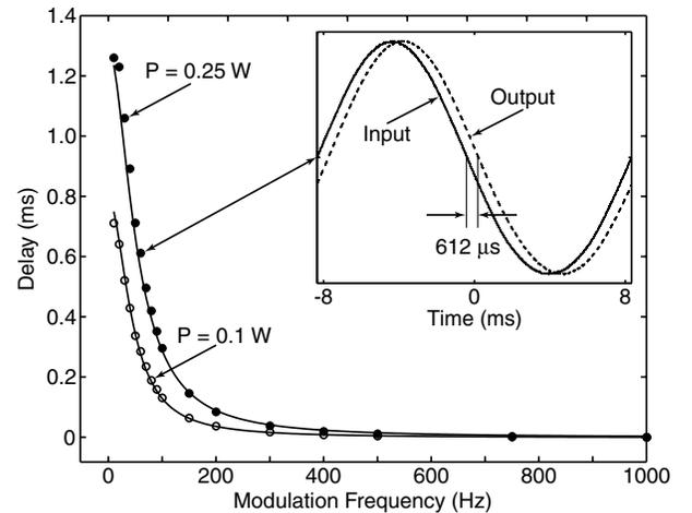
FIG. 3. Observed time delay as a function of the modulation frequency for input pump powers of 0.1 and 0.25 W. The solid lines represent the theoretical model of Eq. (9). The inset shows the normalized 60 Hz input (solid line) and output (dashed line) signal at 0.25 W. The signal was delayed  $612 \mu\text{s}$  corresponding to an average group velocity of  $118 \text{ m/s}$ .
