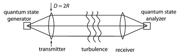
Fig. 1. Schematic of a free-space quantum communication link.
