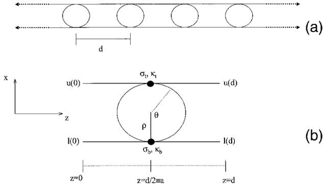
Fig. 1. (a) Schematic of the two-channel SCISSOR. (b) One unit cell of the structure. Filled circles, coupling points at the top and the bottom of the microresonator.
