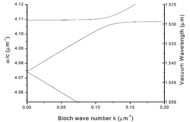
Fig. 2. Dispersion relation for the two-channel SCISSOR with material parameters given in the text. The gap at  $\omega/c = 4.11 \mu\text{m}^{-1}$  is associated with the 59th-order resonance of the microresonator. The gap at  $\omega/c = 4.075 \mu\text{m}^{-1}$  is associated with Bragg reflection. These gaps are at typical communications wavelengths, as indicated by the right-hand axis.
