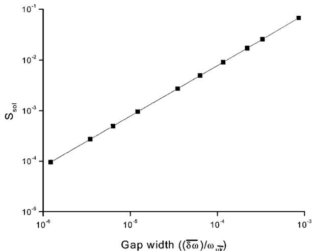
Fig. 3.  $S_{\text{sol}}$  is the ratio of the energy required for forming a gap soliton in a resonator gap to the energy required for forming the same gap soliton in a Bragg gap with the same gap width relative to its center frequency.
