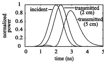
Fig. 4. Ring resonator dynamic transmission characteristics for a 1-ns FWHM Gaussian pulse that is incident upon two distinct fiber ring lengths (2 and 5 cm), corresponding to resonator lifetimes of 1 and 2.5 ns for a resonator of finesse equal to 10.
