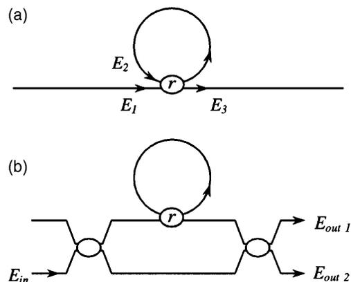
Fig. 1. (a) Nonlinear fiber ring resonator. The circulating power exceeds the incident power by the factor  $(1 + r)/(1 - r)$ , which is very large for  $r$  close to unity. (b) Switching threshold of a nonlinear Mach-Zehnder interferometer can be dramatically reduced by introduction of a nonlinear fiber ring resonator into one arm of the interferometer.
