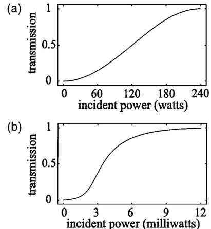
Fig. 3. Transmission characteristics of (a) a standard nonlinear Mach-Zehnder interferometer and (b) the REMZ interferometer of Fig. 1(b). Note that the switching threshold of the REMZ device is lowered by 4 orders of magnitude.
