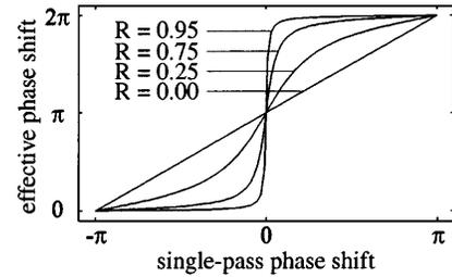
Fig. 2. Effective phase shift  $\phi_{\text{eff}} = \arg(E_3/E_1)$  versus the ring single-pass phase shift  $\phi$  for the fiber ring resonator of Fig. 1(a) for several values of  $R = r^2$ . For values of  $R$  close to unity, the phase sensitivity  $d\phi_{\text{eff}}/d\phi$  can be made extremely large.
