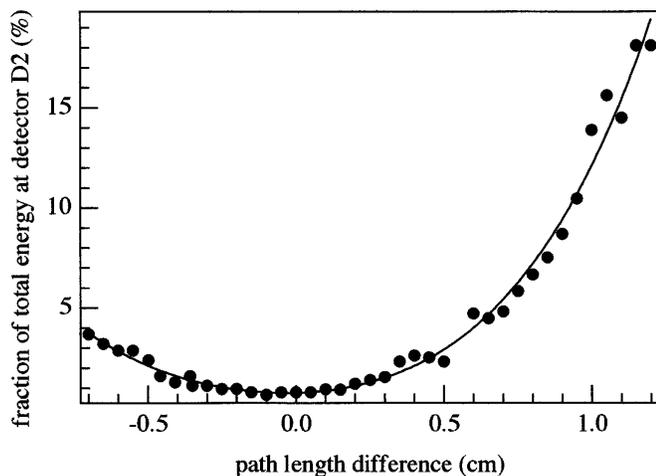
Fig. 4. Fractional depolarization versus the path length difference  $\Delta L_1$  (or  $\Delta L_2$ ). The origin of  $\Delta L_3$  is arbitrary. Note that the amount of depolarization can be reduced to acceptable levels with only centimeter tolerances on the path length difference.
