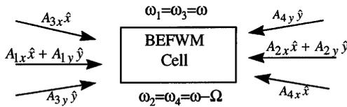
Fig. 1. Brillouin-enhanced four-wave mixing geometry of our experiments. The pump beams are  $A_1$  and  $A_2$ , and the probe beams and their conjugates are  $A_3$  and  $A_4$ , respectively.
