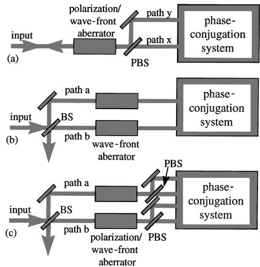
Fig. 2. Several applications of this BEFWM phase-conjugate mirror. For simplicity the pump beams are not explicitly shown. (a) Vector phase conjugation is obtained through use of a polarizing beam splitter (PBS). (b) Beam combining can be implemented as shown, with an ordinary beam splitter (BS). (c) Vector phase conjugation and beam combining are simultaneously produced.
