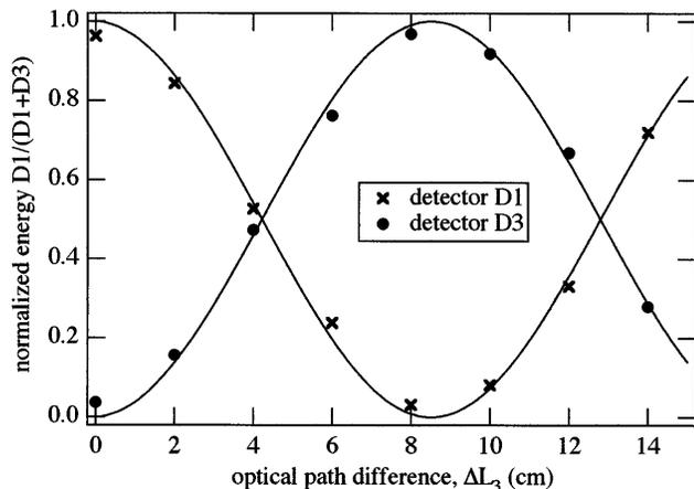
Fig. 5. The return beam can be directed to either D1 or D3 by varying  $\Delta L_3$ . The path length difference need be regulated only to centimeter scale accuracy for nearly complete energy transfer to occur.
