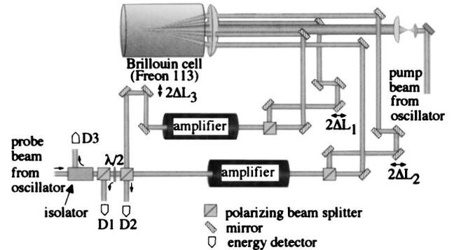
Fig. 3. Laser amplifier system based on the geometry shown in Fig. 2(c). Detector D2 is used to measure the amount of depolarized light, and detector D3 measures the amount of light that is coupled back toward the oscillator. The path lengths  $\Delta L_1$  and  $\Delta L_2$  can be adjusted to control the degree of depolarization while  $\Delta L_3$  is used to adjust the fraction of the output coupled to detector D1.
