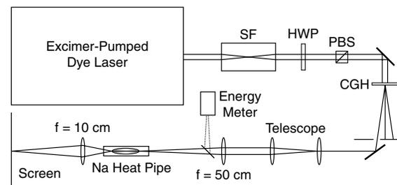
FIG. 1. The experimental setup used to observe filamentation of ring solitons in sodium vapor.
