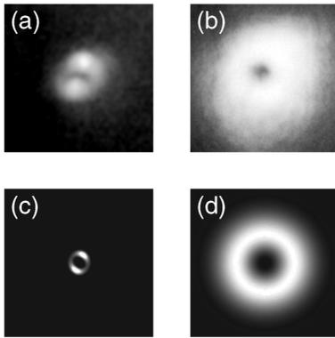
FIG. 2. The experimental output (a) for an  $m = 1$  beam with a pulse energy of 76 nJ breaking into two filaments at a wavelength of 588.950 nm, and (b) tuned far from resonance. In (c) and (d) we show the equivalent results from our computer simulations with parameters corresponding to our experiment and a random 1.5% amplitude noise added to the input beam.
