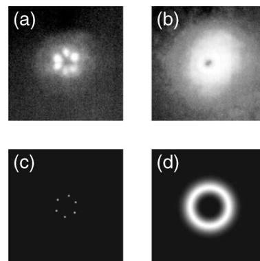
FIG. 4. The experimental output (a) for an  $m = 3$  beam with a pulse energy of 359 nJ breaking into six filaments at a wavelength of 588.943 nm, and (b) tuned far from resonance. In (c) and (d) we show the equivalent results from our simulations.
