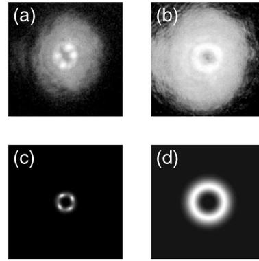
FIG. 3. The experimental output (a) for an  $m = 2$  beam with a pulse energy of 234 nJ breaking into four filaments at a wavelength of 588.943 nm, and (b) tuned far from resonance. In (c) and (d) we show the equivalent results from our computer simulations.
