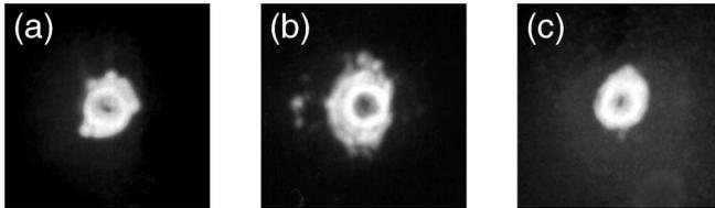
FIG. 5. The beam profile at the output of the sodium cell at higher powers than those used in Figs. 2–4. The tendency of the beam to break into filaments is largely suppressed. (a)  $m = 1$  at  $9.1 \mu\text{J}$ ; (b)  $m = 2$  at  $24.1 \mu\text{J}$ ; (c)  $m = 3$  at  $6.63 \mu\text{J}$ .
