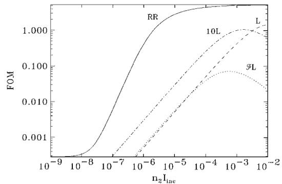
Fig. 2. Comparison of the FOM for the RR with  $\delta\nu = 0$  (solid curve) and nonlinear sections of lengths  $L$ ,  $10L$ , and  $\mathcal{F}L$ .
