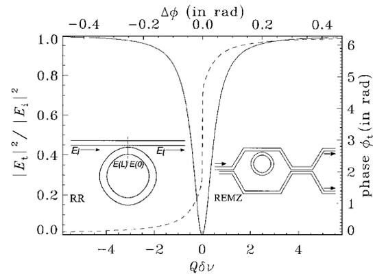
Fig. 1. Squared magnitude (solid curve) and phase (dashed curve) of the transfer function for a single-coupler RR near the critical coupling condition in which the rate of energy coupled into the cavity equals the rate of energy dissipated within the cavity. Insets, RR geometry used for Figs. 2 and 3 (left) and resonance-enhanced Mach-Zehnder interferometer geometry used for Fig. 4 (right).
