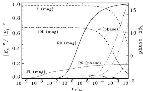
Fig. 3. Intensity transmission (heavier curves) for the RR (solid curves) with  $\delta\nu = 0$  and nonlinear sections of lengths  $L$ ,  $10L$ , and  $FL$ . The corresponding phase changes are shown as thinner curves. The dotted curve corresponds to a nonlinear section of infinite length, which is essentially the same as for a length  $FL$ .
