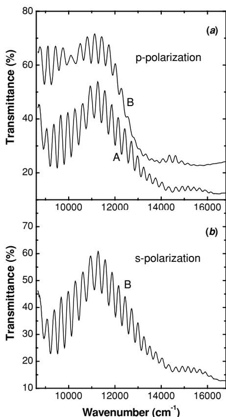
**Figure 4.** Transmittance spectra measured with p-polarized light (a) and s-polarized light (b) at an angle of incidence of  $10^\circ$  (curve A), and  $55^\circ$  (curve B).
