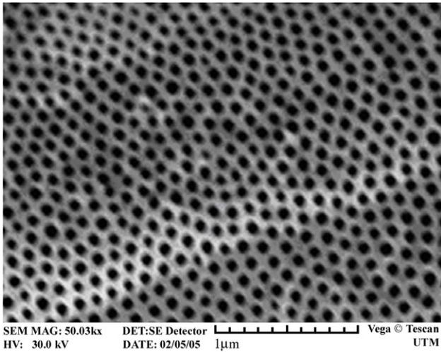
**Figure 1.** SEM image taken from a porous GaP membrane.
