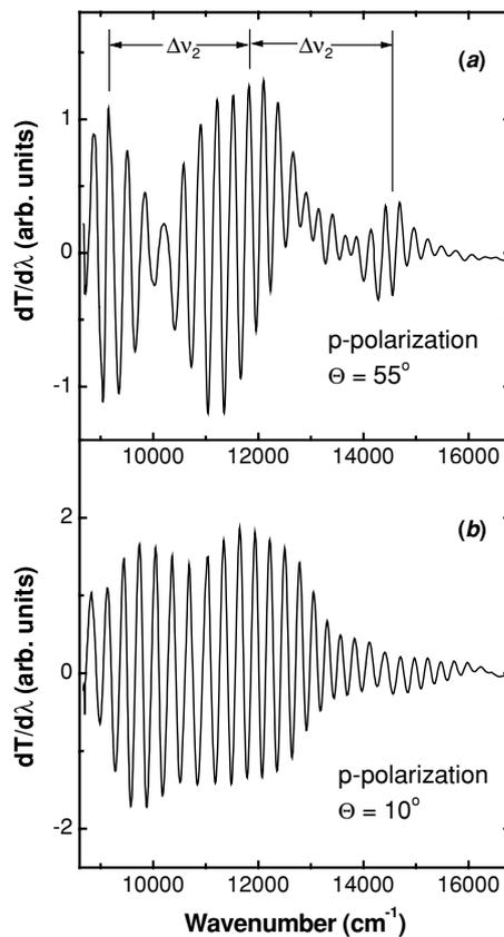
**Figure 5.** Wavelength derivative spectra measured with p-polarized light at an angle of incidence of  $10^\circ$  (a), and  $55^\circ$  (b).
