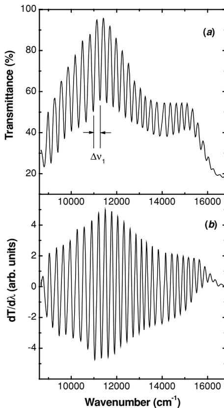
Figure 2. Unpolarized transmittance spectrum (a) and wavelength derivative spectrum (b) measured at normal incidence for an 8  $\mu\text{m}$  thick GaP porous membrane.
