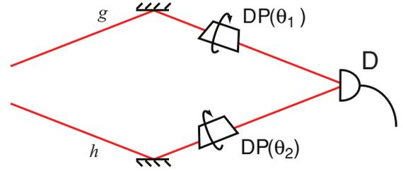
FIG. 2. (Color online) Angular-displacement measurement using  $N$  entangled photons. The photons in modes  $g$  and  $h$  are in the maximally entangled state and have an orbital angular momentum of  $|l\hbar|$  per photon. The detector  $D$  is an  $N$ -photon detector.
