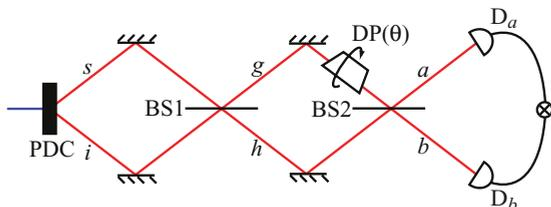
FIG. 3. (Color online) Scheme for supersensitive measurement of angular displacement using entangled photons.  $\theta$  is the angle of rotation of the Dove prism in mode  $g$ .  $D_a$  and  $D_b$  are detectors set to detect photons with OAM mode indices  $\pm l$  only.
