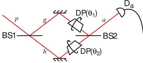
FIG. 1. (Color online) Scheme for angular-displacement measurement using  $N$  independent photons. The photons have an orbital angular momentum of  $l\hbar$  per photon and are detected by the detector  $D_A$  in mode  $a$ . DP stands for Dove prism and BS denotes beam splitter.
