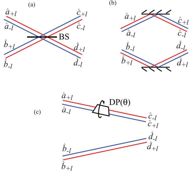
FIG. 4. (Color online) Transformation of OAM modes when they pass through (a) a beam splitter, (b) a pair of mirrors, and (c) a Dove prism.
