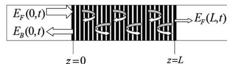
Fig. 6. Schematic illustration of the origin of slow light in a Bragg grating structure. Reproduced with permission from [33].
