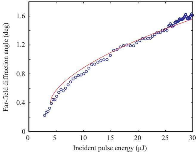
FIG. 3. (Color online) Measured far-field diffraction angle (circles) and the predictions of our theoretical model (solid line) as functions of the incident pulse energy. The square-root dependence on pulse energy predicted by Eq. (4) is evident.
