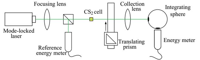
FIG. 2. (Color online) Schematic diagram of the optical configuration used to study the transmission of a 532-nm laser pulse through a 10-mm-long  $\text{CS}_2$  cell.
