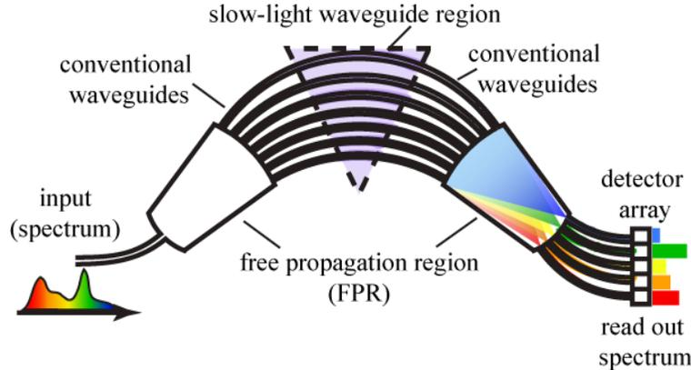
Figure 1. Schematic diagram of a slow-light arrayed waveguide grating spectrometer.
