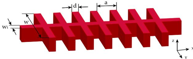
Figure 5. Two-dimensional schematics of a photonic wire with corrugations in the side wall. The length and width of the corrugation is  $w$  and  $d$ , respectively while the lattice constant is  $a$  and the width of the photonic wire is  $w_i$ .
