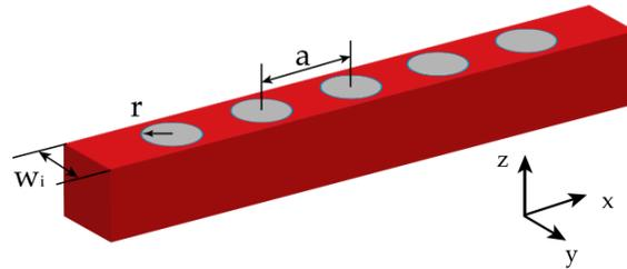
Figure 3. Two-dimensional schematics of a photonic wire waveguide with holes. The lattice constant is  $a$  and the hole radius is  $r$  while the width of the waveguide is  $w_i$ .
