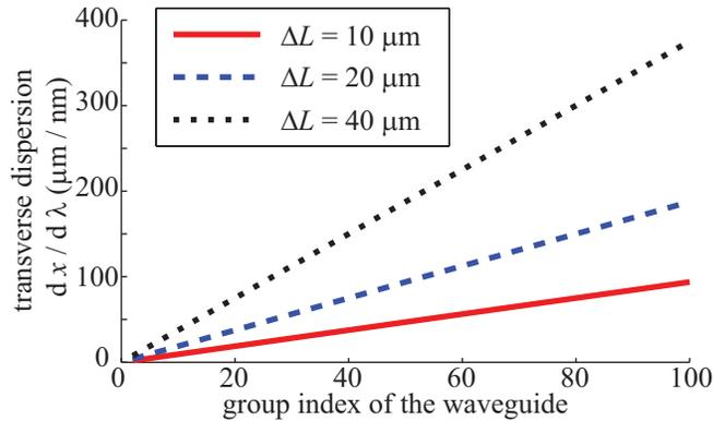
Figure 2. Linear transverse dispersion at the focal plane of the output FPR as a function of the group index of the waveguide of a slow-light AWG with  $\Delta l = 10, 20$  and  $40 \mu\text{m}$ , respectively.
