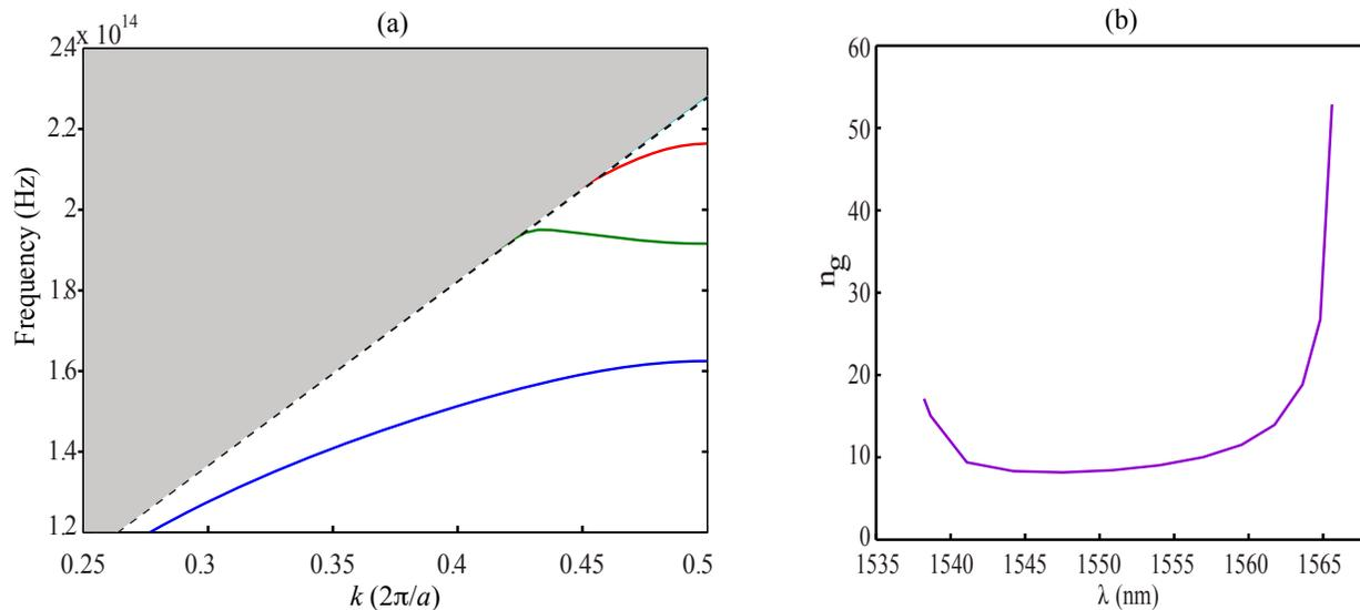
Figure 4. (a) Band diagram for a photonic wire waveguide with holes obtained with  $a = 456$  nm,  $r = 115$  nm and  $w_i = 490$  nm for light transmitted at 1550 nm. (b) Variation of group index over wavelength for the second band in Figure 4(a) in a region around 1550 nm.
