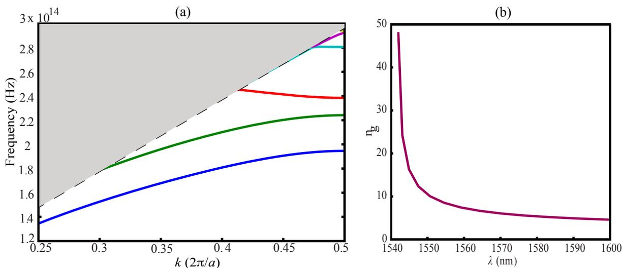
Figure 6. (a) Band diagram for a photonic wire waveguide with corrugations obtained with  $a=350$  nm,  $d=150$  nm,  $w_i=150$  nm, and  $w=850$  nm for light transmitted at 1550 nm. (b) Variation of group index over wavelength for the second band in Figure 6(a) in a region around 1550 nm.
