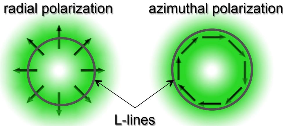
Each has a polarization singularity associated with an intensity null on axis
