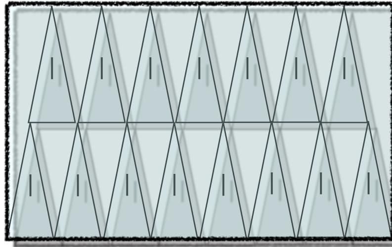
Short lines show the fast axis of the waveplate
