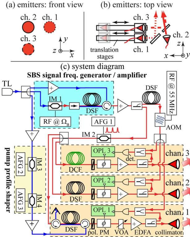
Fig. 1. (Color online) Schematic diagrams of a 2D SLIDAR system, including the top view (a) and front view (b) of the emitter array layout, and the remainder of the system (c). TL: tunable laser, EDFA: Erbium-doped fiber amplifier, OPL: optical phase locking circuit, POL: polarizer, PM: phase modulator, AOM: acousto-optic modulator, VOA: variable optical attenuator, AFG: arbitrary function generator, IM: intensity modulator.
